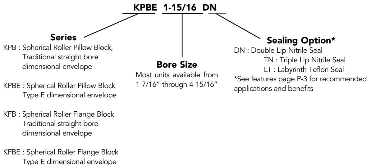
KFB : Spherical Roller Flange Block
