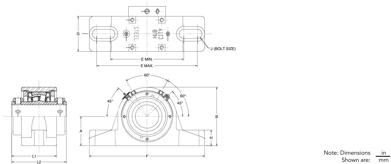
Note: Shaft sizes 2-15/16" and up have a dual locking collar, L2 dimension applies.
