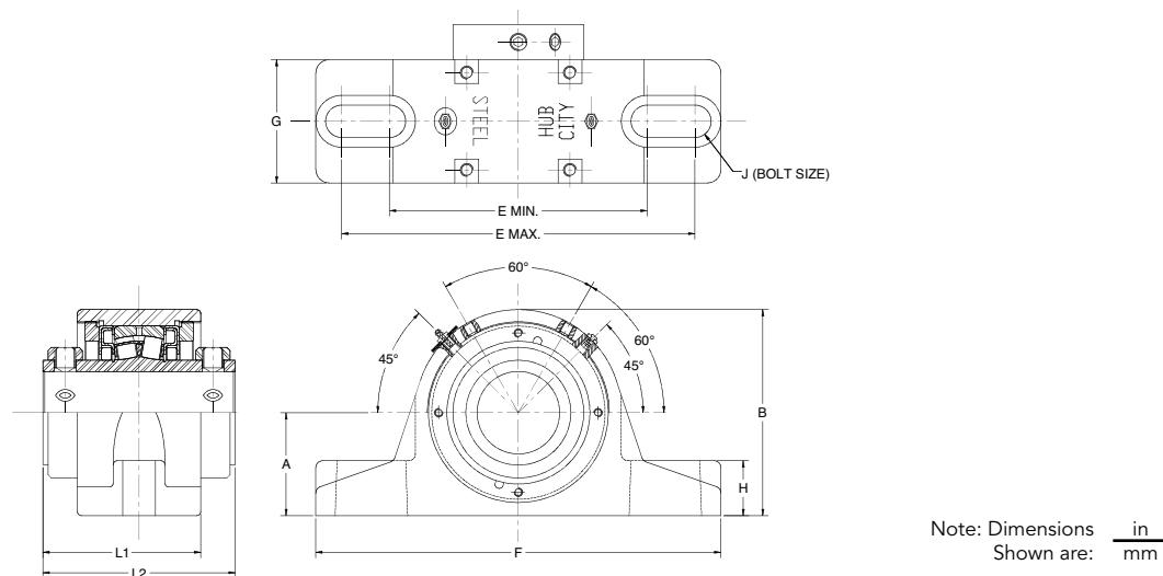
Note: Shaft sizes 2-15/16" and up have a dual locking collar, L2 dimension applies.
